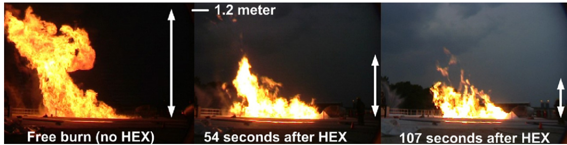
Fig. 11. Pool fire on the 65-m 2 pit before and after foam application rate of 7 L/(min m 2 ).
